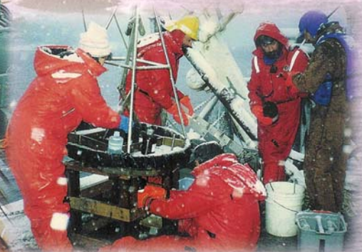
Van Veen Grab sampling for benthic invertebrates and sediment chemistry sampling, Alaska.
