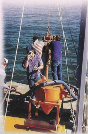
Reverse circulation Vibrolift drilling for mineral sands exploration, Queensland, Australia.
